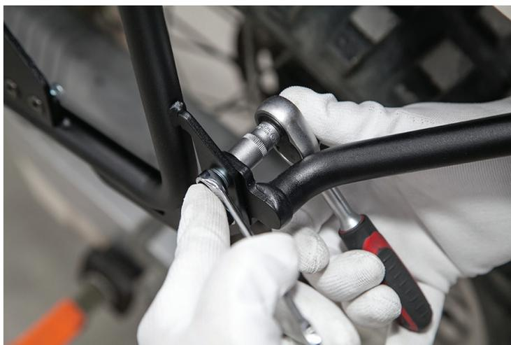
10. Check that all bolts and nuts have been tightened. Double-check again after a test ride.
