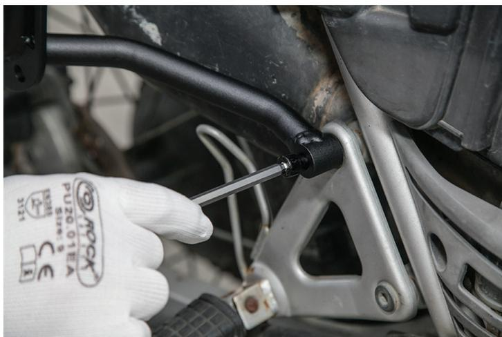
8. Tighten the upper mounting bolts on both sides using a M6 Allen key.
