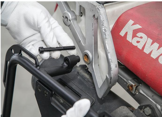
2. Remove the upper foot peg mount bolt and replace it with our supplied M8 Allen bolt while securing the front mount of the pannier rack. Leave it loose.
