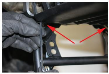
7. Make sure all the bolts are now tightened to the required torque by using a torque wrench!
