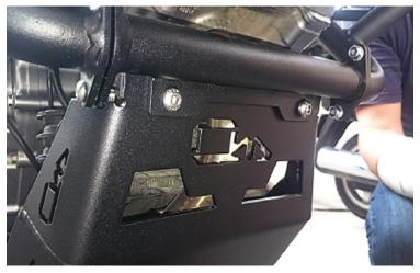
6. Using one hand align the mounting holes on the skid plate and the rear mounting bracket. Insert the M8x20mm (x2) flat head bolts into the holes and tighten both of them to the required torque using a 5mm Allen key.
