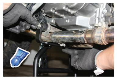
4. Insert the M12x38 (x2) bolts but do not tighten it, yet. Use thread locker!
