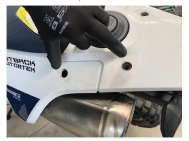
2. Remove the left side factory foot peg using a Torx 40 socket and wrench.
