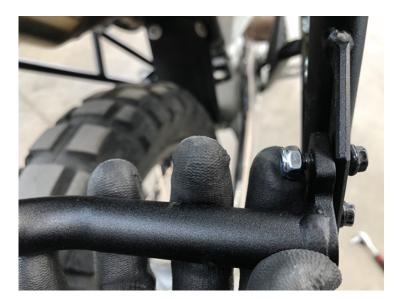
10. Tighten all four nuts by using two 10mm wrenches and/or 10mm socket and ratchet.
