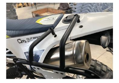
4. Insert the supplied M8x40mm bolt through the front tab and the M8x35mm bolt through the rear. Use T30 torx socket. Only one or two turns to keep both bolts loose.
