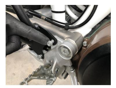
8. Mount the rear cross brace. Please make sure that the cross brace's tabs end up between the pannier frames' tabs.
