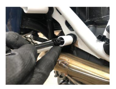
6. Remove the lower factory Allen bolt on the right side of the motorcycle.
