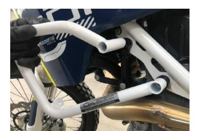
4. Insert the supplied M10x30mm bolt on the top. Only one or two turns to keep the bolt loose.
