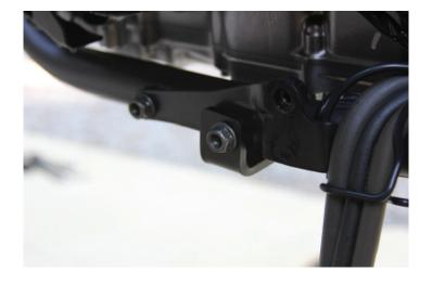
4. Mount the skid plate. First insert the two M8 button head Allen bolts with the washers, handthread and gently tighten using a 5mm Allen key or 5mm Allen socket. Leave it loose.
