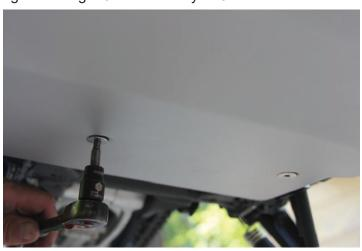
6. Tighten the skid plate mount bracket bolt now using a 12mm socket and ratchet. Factory recommended torque specs 44Nm.
