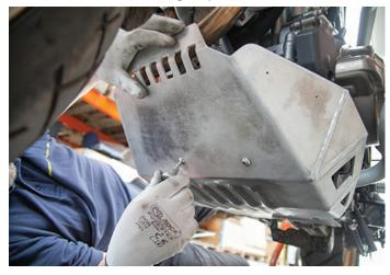
8. Insert and hand-thread the M8x12 mm Allen bolts after lining up the rear mouting holes.
