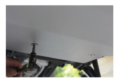
7. Finally, go ahead and tighten all the bolts and nuts to the required torque specs and make sure to check again after going out for a test ride.
