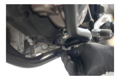
6. Move onto the right side (exhaust side) of your Africa Twin. Look underneath the bike. There are two through bolts in the frame.
