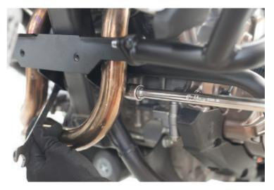
15. Final step: make sure to tighten all the bolts and nuts to the required torque specs. This step includes the crash bars' bolts and nuts as well. Important: check every bolt and nut again after riding at least 150kms/100miles.
