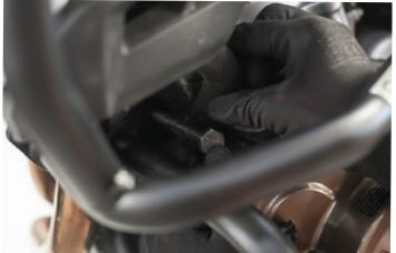
4. Mount the counterpart of the clamp on the reinforcement bar. Insert the two supplied button head Allen bolts. Place on the washers and hand-thread the nyloc nuts.
