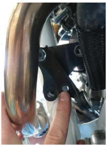
5. On the left side, behind the tool box push on the tab slightly with your fingers to create some space for the crash bar's rear mounting tab. (Step #13).
