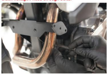
6. Remove the three bolts on the rider's right side. Use a 12mm socket, extension and ratchet.
