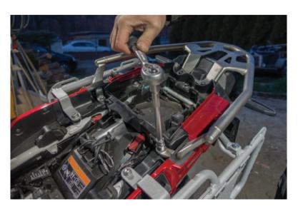
22. Finally tighten all the bolts and nuts. Make sure to double-check all the bolts and nuts once again after a test ride.
