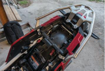
3. Remove the two Allen bolts that keep the plastic cover in place above the rear brake light.
