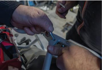
19. After lining up the mounting holes of the rear cross brace, go ahead and insert the 6x20mm hex head bolts and secure them using the provided washers and locking nuts.
