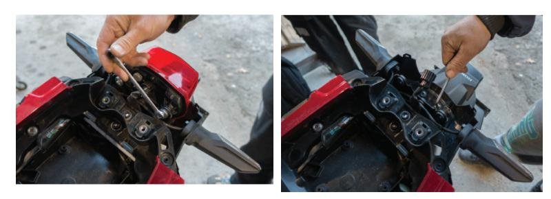
7. Using 12mm socket and wrench, remove the top bolt from the middle in order to drop the license plate holder.
