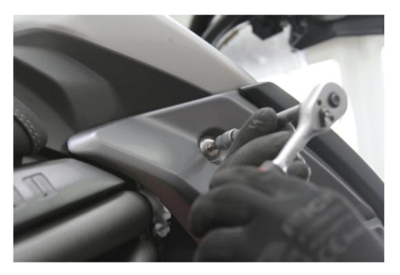
7. Remove side panels gently. No need to disconnect the turn signals but make sure to use a string to loosely hang both side panels on the side of the bike.
