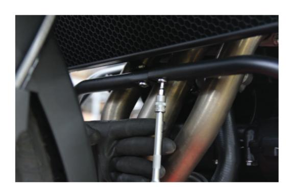
10. On the right hand side begin removing the engine through-bolt. Necessary tools: two ratchet, one short and one vey long extension (12" or 30cm), M8 Allen socket (XC/XR), T50 socket torx (XCX/XRX) and one universal joint.
