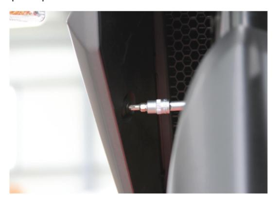
4. Using a 5mm Allen kepremove the upper bolts. Again, from both right and left sides.
