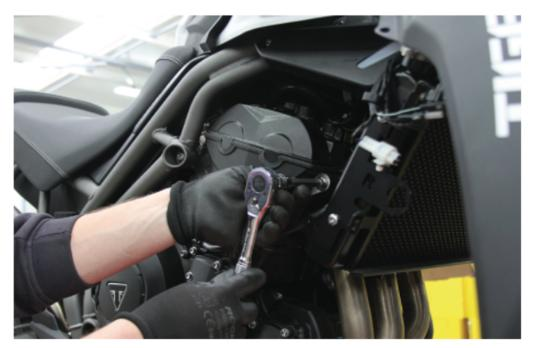
11.Using a T50 torx or 8mm Allen socket, universal joint, long extension and ratchet begin removing the through bolt.
