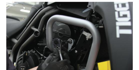
14. Insert the two M8 Allen bolts through the crash bar's lower mounting tab, thus connecting it with the engine guard. Put one washer on each of the two bolts and thread on the nyloc nuts.
