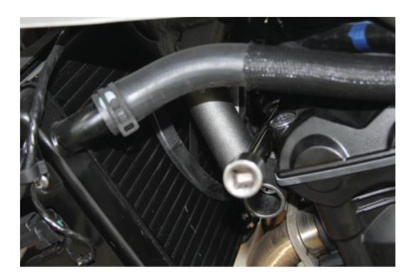
12. Mount the engine guard on the right hand side. Make sure to use thread-locking fluid (blue) and leave all three bolts loose.
