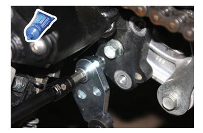
3. Place the right mount (with spring post) on the frame with the bumpers (wheels) facing out and thread the M10x40mm into the hole using an 8mm Allen key. Don't fully tighten it yet.
