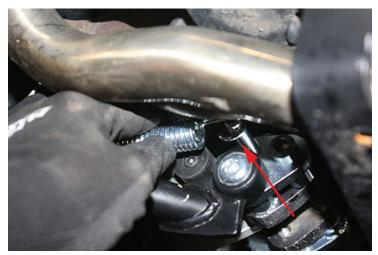
7. Using a long-nose plier, hook the other end of the small and big spring onto the center stand spring post. Make sure all four hooks are properly and securely placed onto the spring posts
