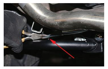
8. Finally insert the M10x30mm (fat head) bolt on the left side (rider's left) and tighten it to the required torque specs. Use threadlocker!
